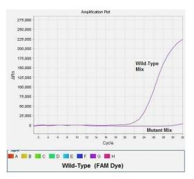
Amplification plots of mutations can be analysed by related dye\*. The CT value should be between **21 \leq CT \leq 26**. These values are optimised according to the SNPure<sup>®</sup> Blood DNA Isolation Kit and MN NucleoSpin <sup>®</sup> Blood DNA Isolation Kit. CT values may vary  $\pm 2/3$  cycle according to the DNA isolation protocol.
